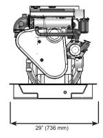
M944T Overall Dimensions L x W x H: 60.0 x 29.0 x 30.5 inch (1524 x 736 x 775 mm) Sound Enclosure Dimensions L x W x H: 60.0 x 29.0 x 32.0 (1524 x 736 x 813 mm) Sound Enclosure Weight: 140 lbs. (64 kg)
